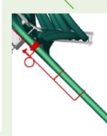
**PENDITWIST MODELS Hose-holding springs** for direct in-line spreading on the ground.
